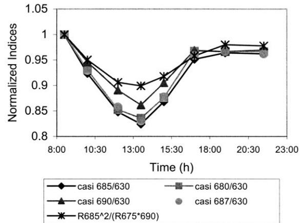
Figure 5. Comparison of R685/R630, R690/R630, R680/R630, R687/R630, and R685<sup>2</sup>/(R675·690) normalized to the first measurement for comparison purposes. R685/R630 varies up to 17% during the day, while the percentage variation of R685<sup>2</sup>/(R675·690) is 10%. All indices show similar behavior as expected for changes in the 680–690-nm region due to fluorescence.
