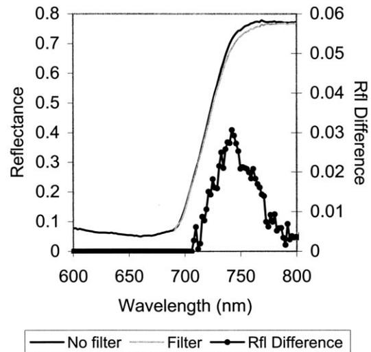
Figure 1. CASI canopy reflectance measurements of *Acer saccharum* M. seedlings in laboratory. Data were collected from the plant material using the Schott RG695 filter with dark-adapted plant material and then without the filter, thereby allowing red light to reach the plant material. A reflectance change in the 730–750-nm range can be detected due to the photosystem excitation by red light. The maximum reflectance difference of 3% is observed at 742 nm.
