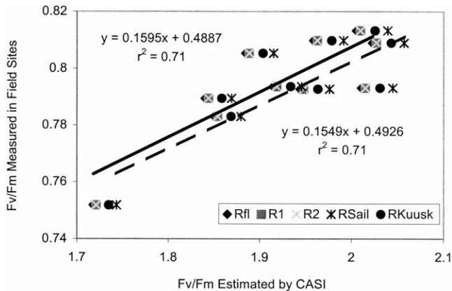
Figure 9. Estimation of Fv/Fm from CASI data using the R683<sup>2</sup>/(R675-R691) algorithm developed at leaf level (Rfl) through R<sub>∞</sub> (R1 and R2) and CR (SAIL and Kuusk) simulation models (RSAIL and RKuusk). The data correspond to *Acer saccharum* M. study sites. Estimations are not affected by the simulation approach whether the optical index is calculated using R<sub>∞</sub> (dashed line) or the canopy reflectance (CR) models (solid line).
