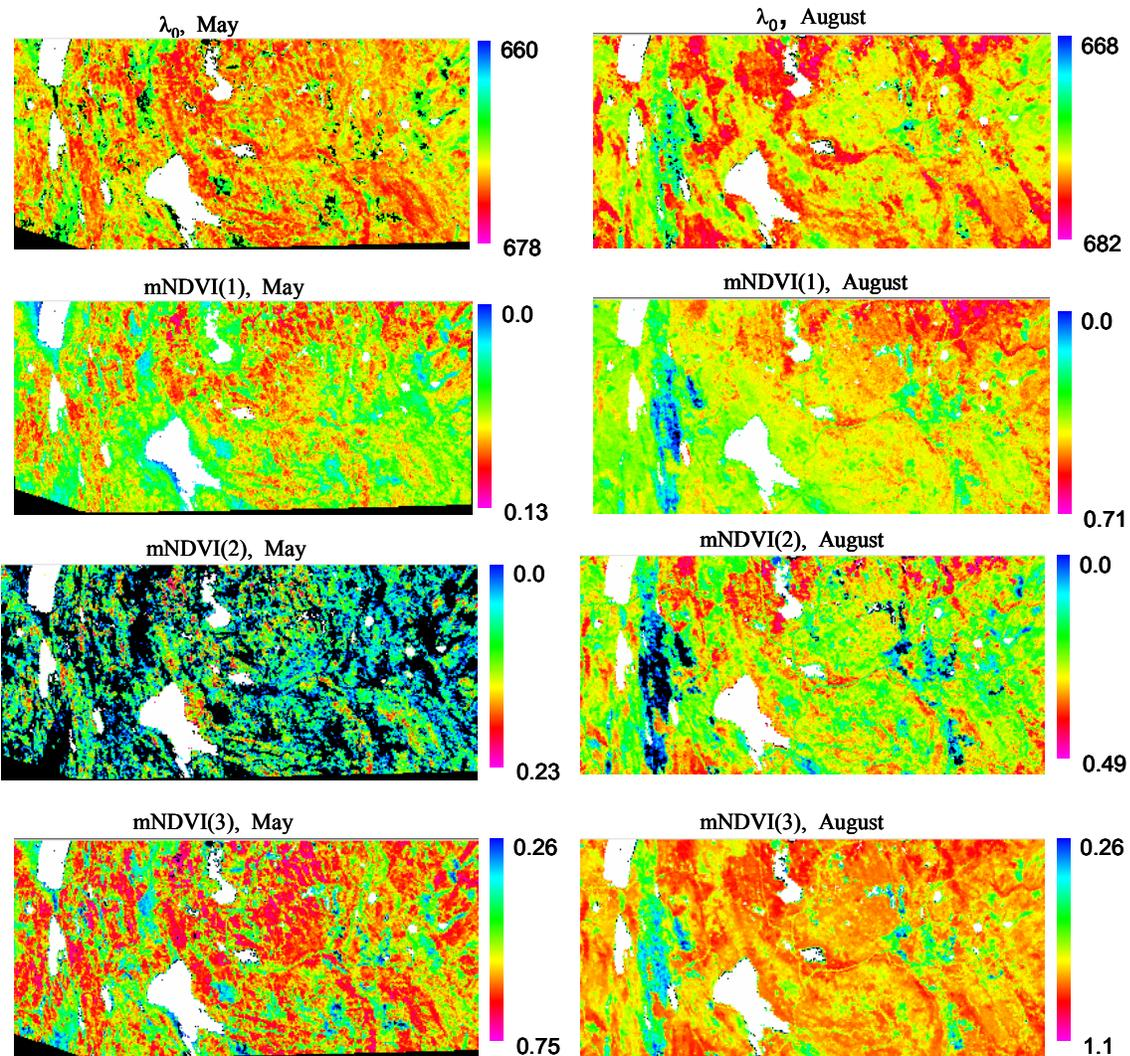
Fig. 6 The images of optical indices calculated from MERIS reflectance data in May and August, where the white areas are water bodies. Please note that the scale is varied.
