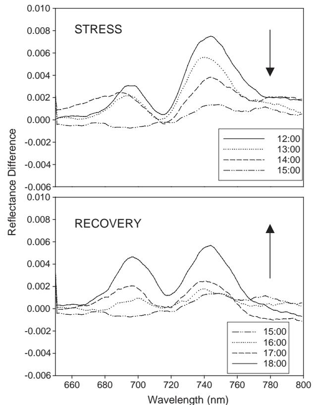
Fig. 4. Difference spectra calculated for day 1 showing a reduction in steady-state chlorophyll fluorescence as heat stress develops mid-day followed by an increase in steady-state chlorophyll fluorescence during the recovery period.
