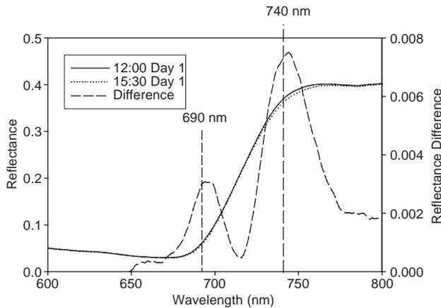
Fig. 3. Difference spectrum between unstressed (1200 h) and stressed (1530 h) canopy reflectance measurements showing the contribution of steady-state chlorophyll fluorescence to apparent reflectance. Note that the emission maxima for chlorophyll fluorescence are centered at 690 and 740 nm and coincide with the maximum reflectance difference values.
