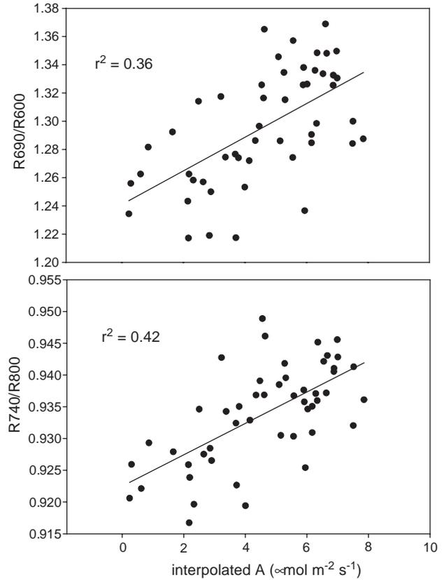
Fig. 7. Scatter plot of the relationship between the fluorescence ratio indices (FRI) and interpolated  $CO_2$  assimilation rates. Plot includes measurements taken every half hour over the course of the 4-day experiment.
