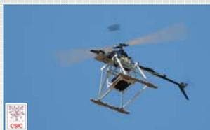
Figure 1: Quanta-H, is a rotary wing UAV of 1.9 m main rotor diameter capable of carrying 7kg of payload.
