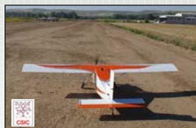
Figure 2: Quanta-G is a fixed wing UAV of 3.2m wingspan with an endurance of 30 minutes flying at 90km/h and available payload of 5.5kg.
