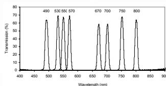
Figure 3: Spectral characteristics of some of the filters used on the multispectral camera.
