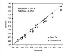
Figure 5: Field validation of the surface temperature. The plot shows the result with and without atmospheric correction.
