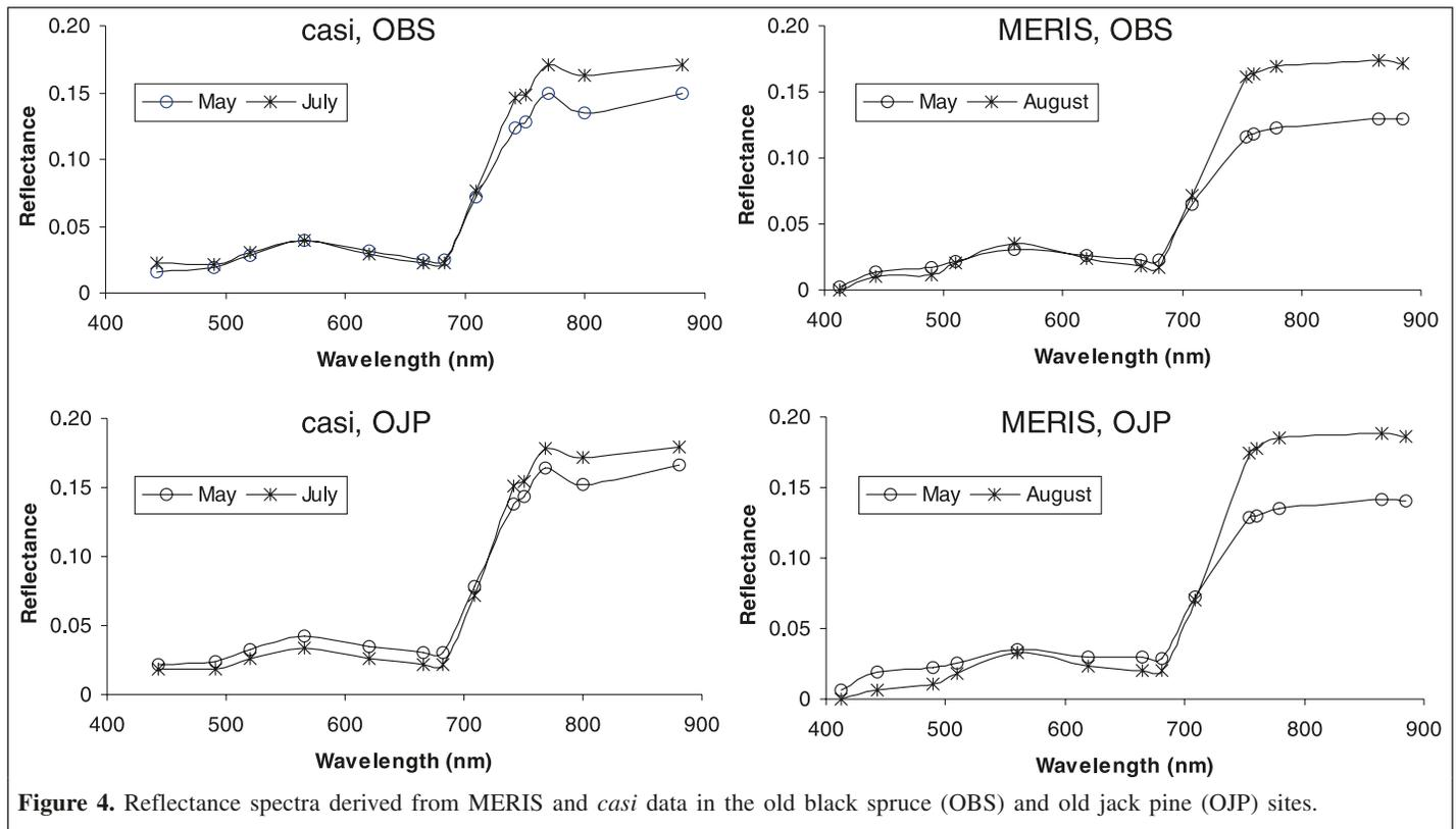
**Figure 4.** Reflectance spectra derived from MERIS and *casi* data in the old black spruce (OBS) and old jack pine (OJP) sites.
