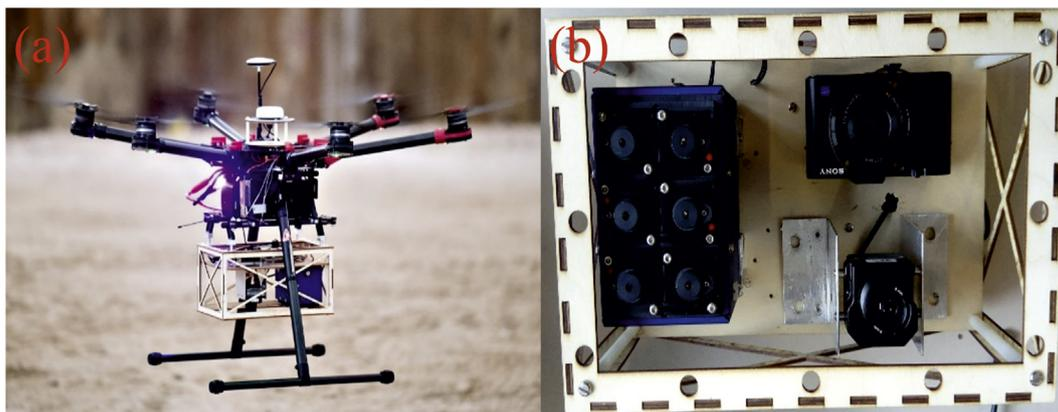
Fig. 2. (a) DJI S900 vehicle platform and (b) the payload including an RGB camera, a thermal infrared camera and a multispectral camera.
