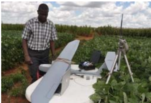
Skywalker complex aerial phenotyping platform, a remote-controlled plane provided with an advance flight system.
