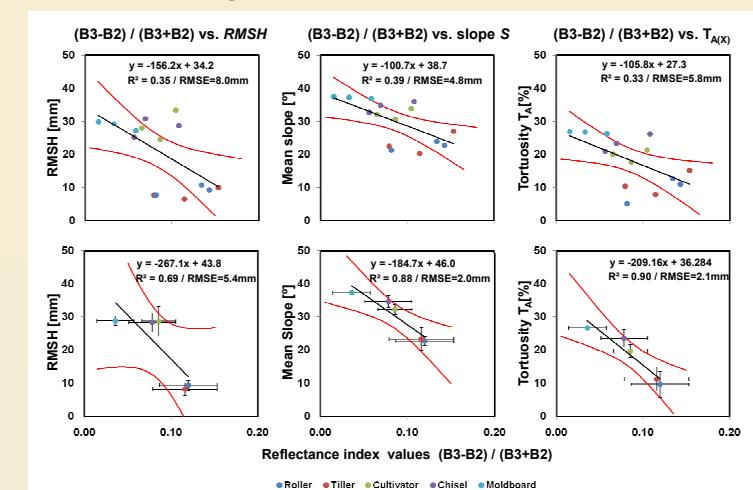
**Figure 5:** Regression models for reflectance index  $(B3-B2)/(B3+B2)$  from 8:30GMT imagery data. Only models for three roughness indices are shown. Upper row are models using single plot data, lower row are based on group means of tillage treatments.
