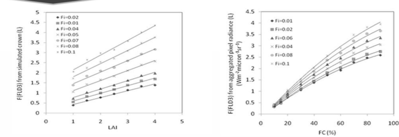
FluorFLIGHT, a modified version of the 3-D radiative transfer model FLIGHT was developed to enable the simulation of canopy radiance and reflectance including fluorescence effects from different spatial resolutions and percentage cover levels. The FluorFLIGHT model was specifically developed to assess the sensitivity of the fluorescence signal on heterogeneous forest canopy images.
