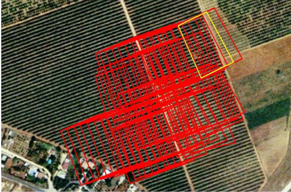
Figure 1.9. Footprints for the images acquired during a flight plan conducted over an orange orchard. Red rectangles correspond to single image frames. The yellow rectangle represents the overlapping of two consecutive images (stereo-pair).
