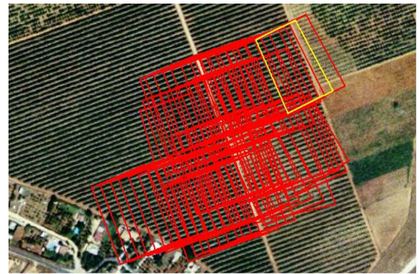
Fig. 9. Footprints for the images acquired during a flight plan conducted over an orange orchard. Red rectangles correspond to single image frames. The yellow rectangle represents the overlapping of two consecutive images (stereo-pair).
